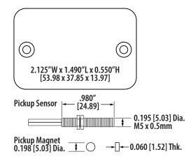
Included: GDI MotorTACH RPM pickup Sensor Motor shaft magnet disc
