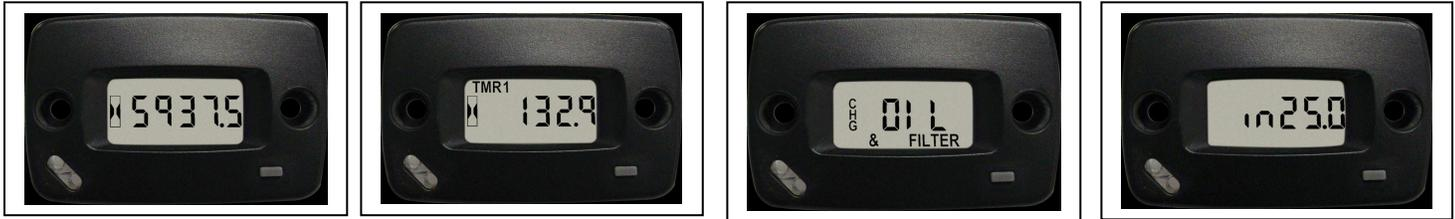
**GDI Vibration Activated hour meters are the solution for monitoring equipment run time without including road travel\*. The meter is wireless and simply mounts on any equipment that requires monitoring of run hours, maintenance service reminders, cycle counting, and timers. This product is perfect for equipment without power, or where wiring is not feasible. Knowing equipment run time, what to service and when to service is the key to a successful maintenance program!**
