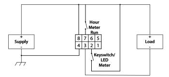
Example 1: Hour Meter switched count enable & separate switch for LED bar light enable. Includes load shutdown.
