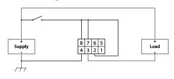
Example 2: Single switched Hour Meter count enable & LED bar light enable. Includes load shutdown.
