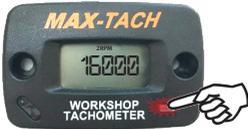
Hold down button for 3 seconds to view MAX RPM
